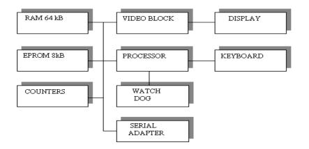
Fig.7. The block scheme of SAPI-02
